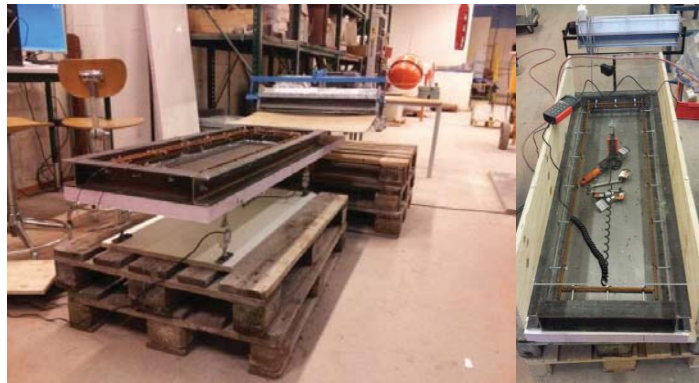
Figure 1 – Test setup for plastic shrinkage crack experiments at LTU.
