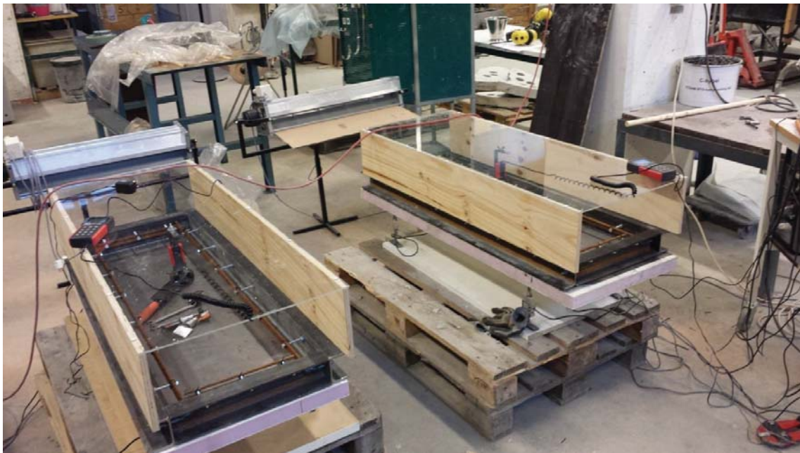
Figure 3.1 – Two rectangular mould test setups with fans and Plexiglas wind tunnels, placed on four load-cells.
